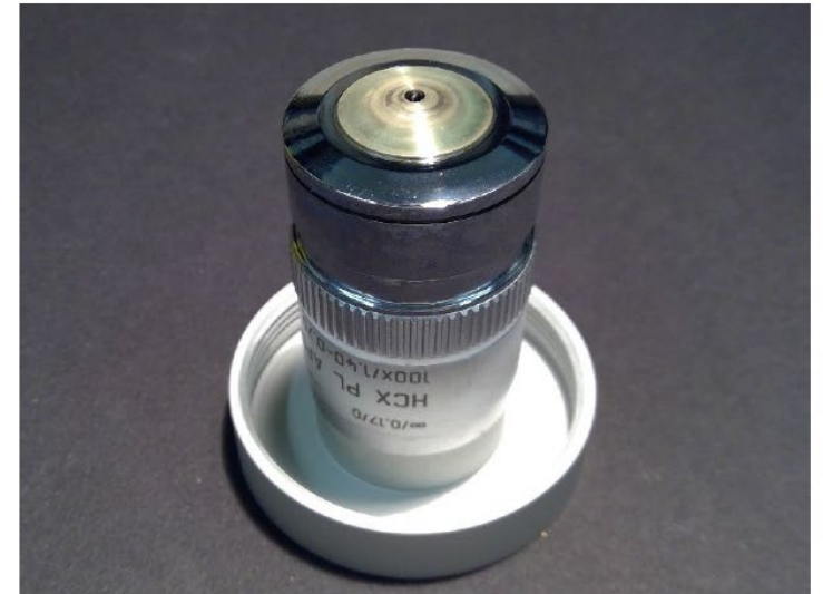
Fig. S9 | Photograph of the used microscope objective lens with applied photoresist for dip-in 3D laser nanoprinting. For dip-in 3D laser nanoprinting, the amount of applied photoresist is on the order of a few microliters. Therefore, the photoresist cannot be seen on this photograph. Note that the bronze colored disk on top of the microscope lens is not the photoresist, but part of the objective lens metallic body.
